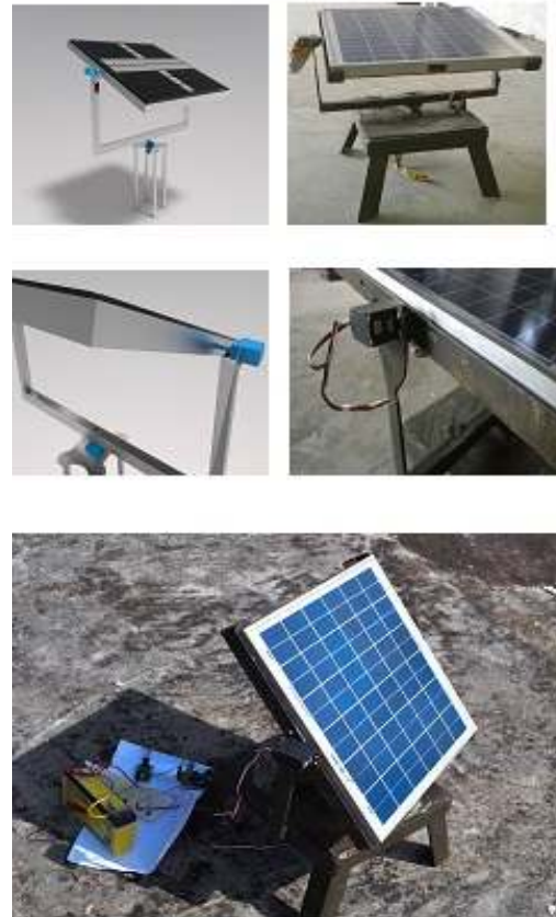
Figure-4: Solid works model & Practical model showing horizontal & vertical motor
