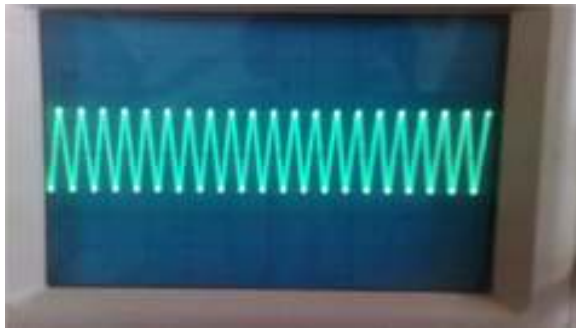
Fig 5.3: Output signal from APR9600 (carrier) [x-axis = 5\mu\text{s} , y-axis = .5\text{V pp} ]
